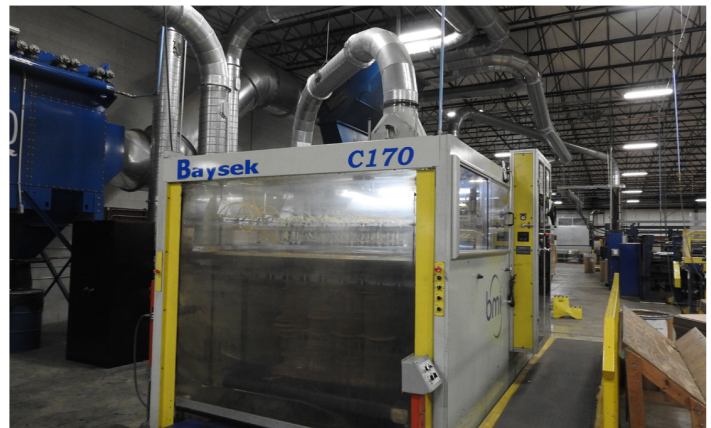
Arrow Carton's Baysek C-170 diecutter has become the 'work-horse' of Arrow Carton's converting machinery.
