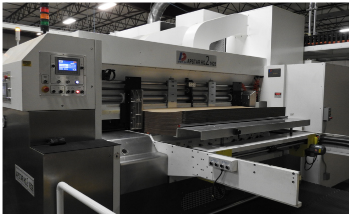
Arrow Carton added a Haire Group Apstar 2-color flexo folder gluer two years ago.
